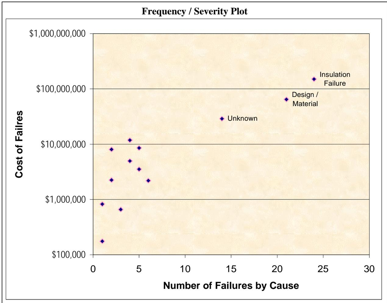
Figure 1 – Frequency - Severity of Transformer Failures
